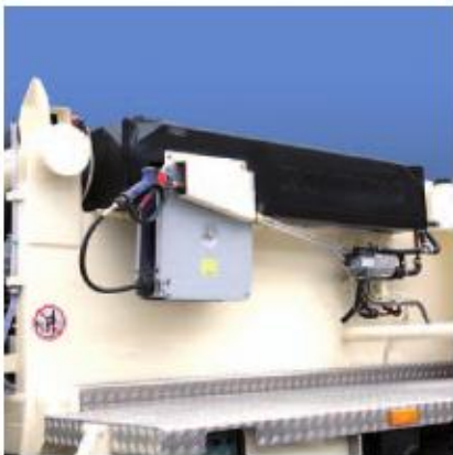
A 600 litre water tank placed directly behind the hopper that can be equipped with a water heating system and the optional high pressure pump and cleaner.
