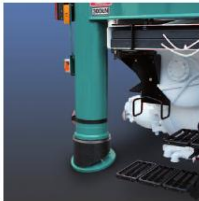
The front and rear outriggers come with attached swivel pads.
