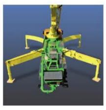
The outrigger forces are passed to the torsion resistant base frame over a broad surface area, giving this machine a solid stand during pumping operation.
