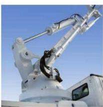
The spacious turret gives good accessibility to the pipeline or hydraulic lines for easy maintenance.
