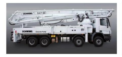
The overhead roll and fold distributes the load evenly onto the 4 axles and that without any overhang on the S 46 SX. The large water tank in the rear outrigger, and ample stowage room complete the specs of this operator friendly machine.
