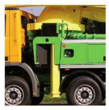
All outrigger cylinders operate in a protective tube system. This protects then against mechanical damage and they are not exposed to buckling forces.
