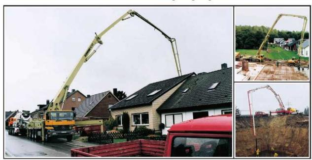
single-sided set-up for fail-safe operation when the pump can only be stabilized on one side. An absolute must for machines that need
