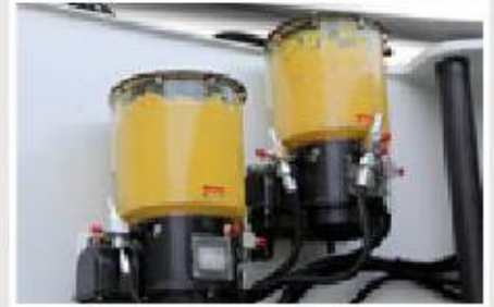
Central greasing system
