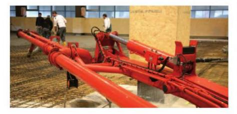
In the working position the extended cylinders are on the top of the boom. This protects them from collision and concrete spills. In the working position the extended cylinders are on the top of the boom. This protects them from collision and concrete spills.
