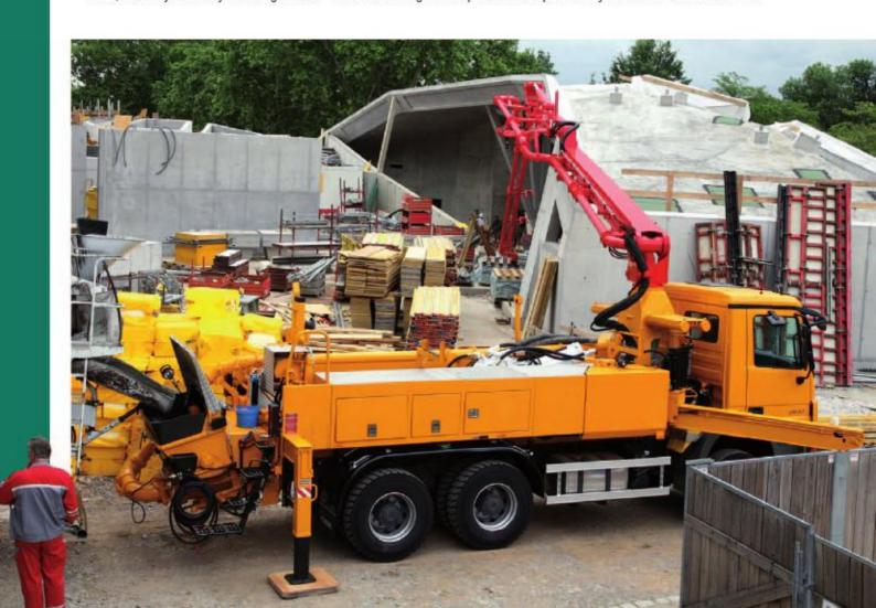
The machine is equipped with removable hose boxes, enabling the operator to use it as a fully functional refurbishment pump.
