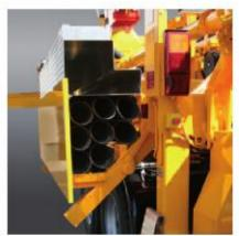
The hydraulic hose box can be lowered without outriggers down and putting the hoses within easy reach of the operator.
