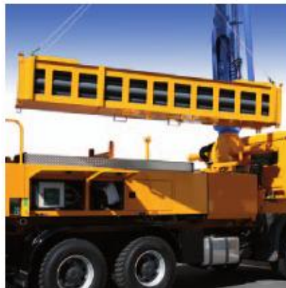
The hose storage boxes on the right side can be loaded and unloaded by a fork lift, crane or the pumps own boom.
