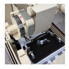
The outstanding accessibility to the water box allow a fast and easy piston change. The integrated water box flushing system minimizes the daily cleaning procedure.
