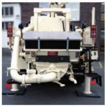
The turnable outlet is an option that allows the operator to connect the pipes to both sides, expanding the scope of his applications.
