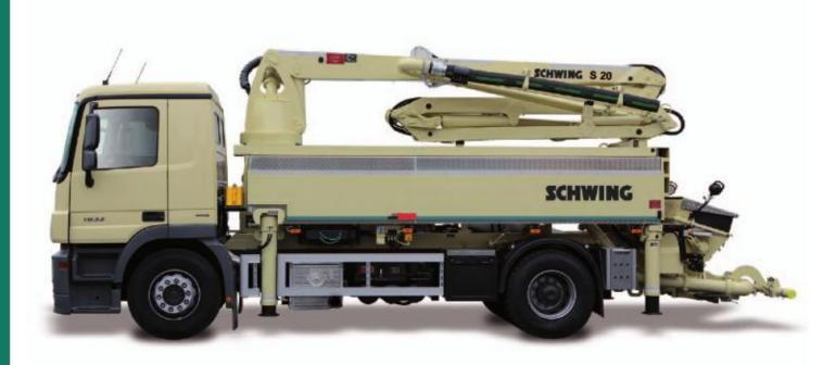
Permanently mounted hose boxes ensure convenient access to 100 m of hose up to DN 75 on the left side and 36 m of hose up to DN 100 on the right side.
