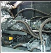
The hydrostatic drive features rugged, sturdy axial-piston pumps with power regulator and additional output adjustment.
