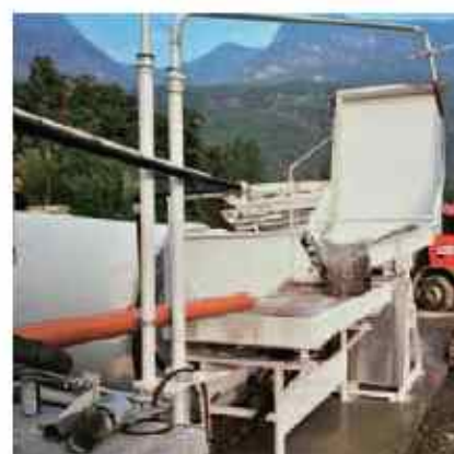
Hydraulic skip for feeding surplus materials from concrete pumps; 1,100 liter capacity.
