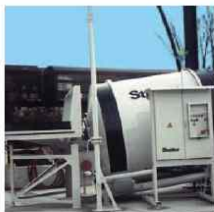
Alternatively, a semicircular feed hopper with a 2.5 m width is available for the RA 12/20.
