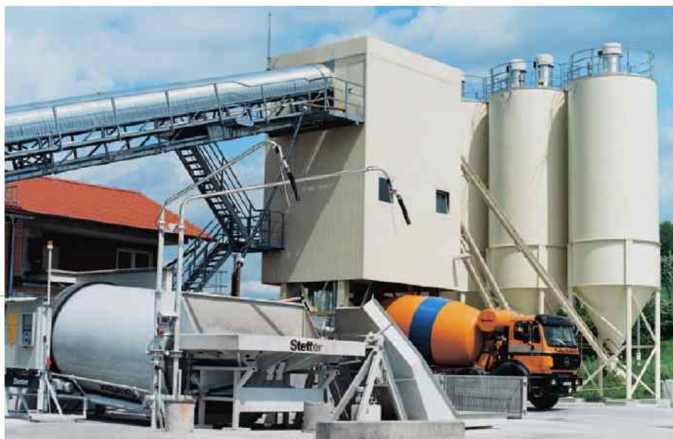
The RA 20 with square feed hopper, width 3.2 m, two water booms and optional hopper.
