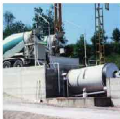
Inground design with ground-level feed height.
