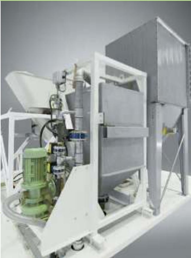
A logical development in combination with recycling plants: hot-galvanized water weighing container for weighing of fresh water and residual concrete slurry water. The weighing system can be combined with a slurry water pressure pump. Water is then led into the mixer via spiral nozzles.
