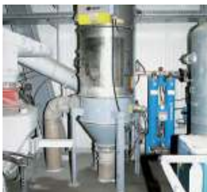
In order to keep the mixing plant's platforms free from dust to a large extent, a forced dedusting device can be installed.
