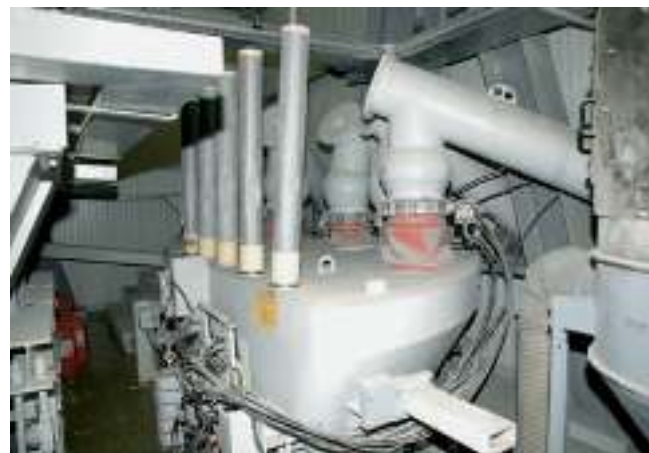
The cement weighing system is equipped with load cells. ■ The inside of the weighing container is protected with durable sliding means. ■ The standard equipment comprises six inlets (upon request up to nine) and a vibrator. ■ If white cement is used, a second weighing system will be installed. ■ The de-aerator provides optimal dust protection. ■ Weighing systems with two mixers are equipped with a two-way distributor.
