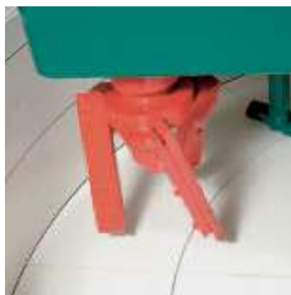
The agitator achieves the highest concrete homogeneity and the most effective breakdown of cement paste.
