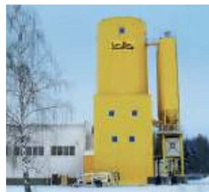
Thermal insulation of mixing and weighing platform is done with sandwich or profiled plates/mineral wool/smooth plates. The section \pm 0 up to the lower edge of the platform can optionally be covered. For thermal insulation of the aggregate silo profiled plates/mineral wool will be used.
