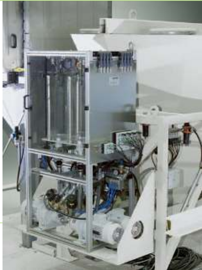
Where flowmeters or volumetric batching devices were used for batching of admixtures, Stetter nowadays installs weighing systems with fully automatic flushing. Size and number of compartments as required.
