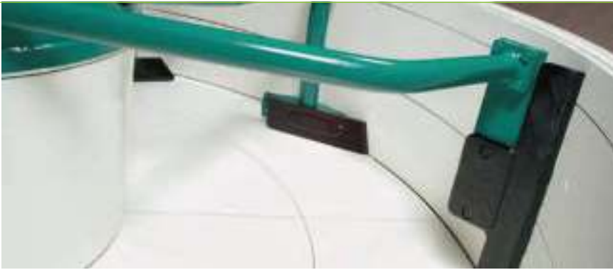
Pictures top left and right: the inner and outer scraper support mixing and discharging effect.
