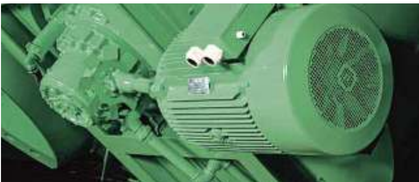
The drive with planetary gear and flange-mounted hydraulic pump.
