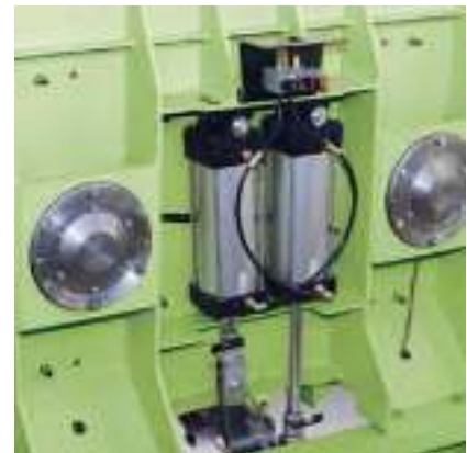
The pneumatic discharge gate operation.
