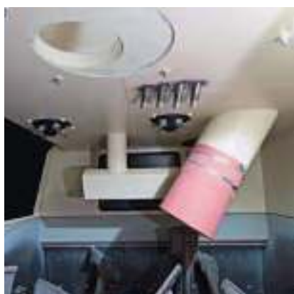
Nozzle heads for cleaning of the mixer.
