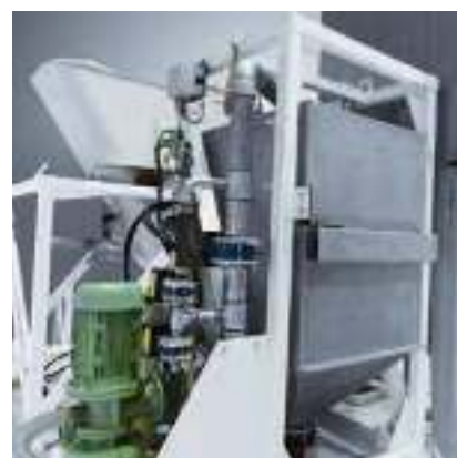
Water weighing system with discharge pump for pressurised feeding of water into the mixer.
