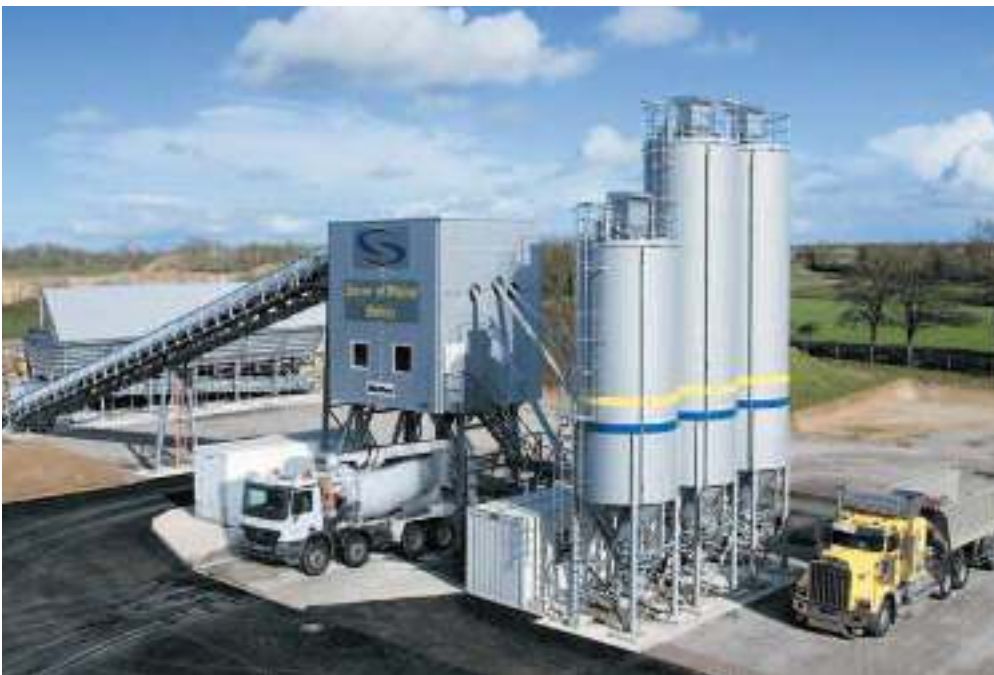
HN 1.5 with pan mixer, capacity 78 m 3 /h compacted concrete.
