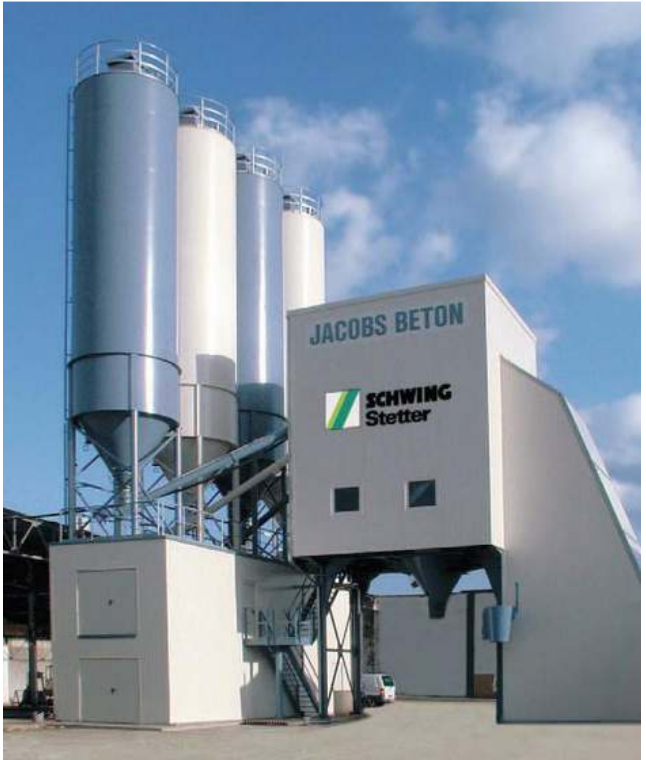
HN 3.0 with twin-shaft mixer, capacity 120 m 3 /h compacted concrete.
