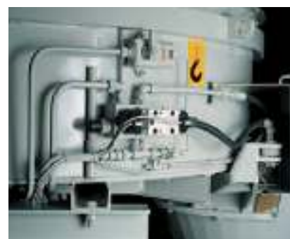
Manual emergency emptying
